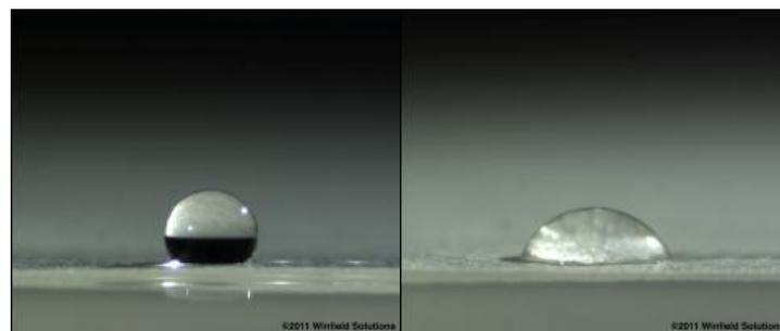
Photographs illustrating water surface tension without (left) and with a nonionic surfactant (right).
