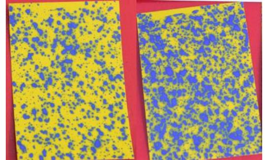
Photographs illustrating coverage differences between 10 GPA (left) and 20 GPA (right) with the same nozzle.
