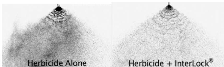
High speed photography from WinField United wind tunnel without (left) and with a deposition aid (right).
