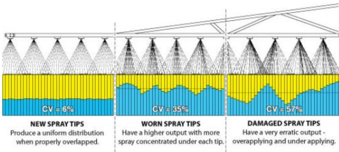
Figure illustrating variation between individual nozzles. (Image source, Tee Jet).
